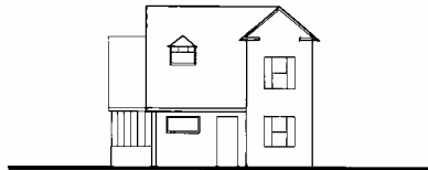
Compatible contrast: addition is different than original structure, however it is compatible; the original structure retains its presence.
