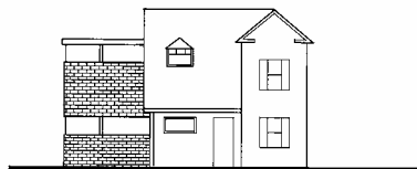
Incompatible contrast: addition is too contrasting; draws attention; compromises integrity of original building.
