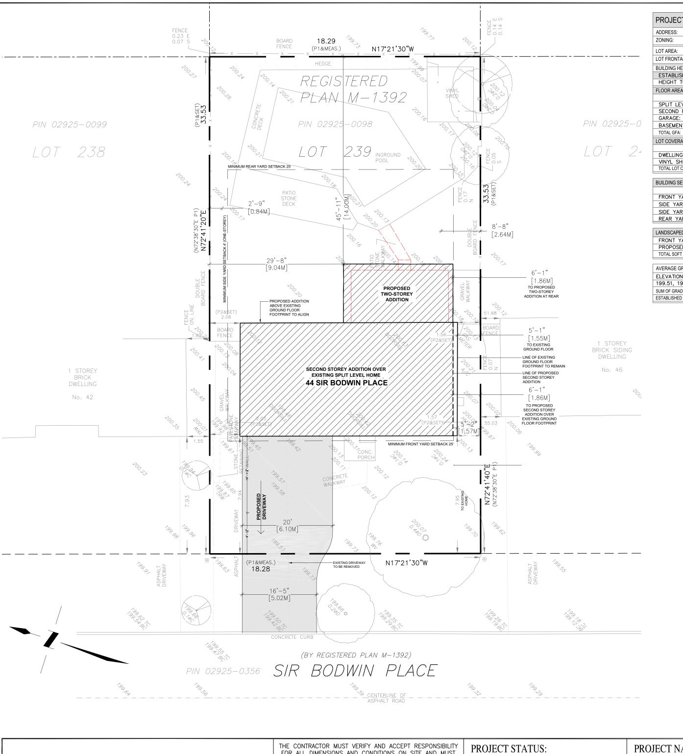
PROJECT STATISTICS 44 SIR BODWIN PLACE, MARKHAM, ON L3P 2X8 613.58 sq.m LOT FRONTAGE: 18.28 .m BUILDING HEIGHT (MAX 9.8m) ESTABLISHED GRADE: 199.89 m HEIGHT TO HIGHEST RIDGE: 8.88 m FLOOR AREA (MAX 45%) - PROPOSED NET FLOOR AREA = 50.4% EXISTING PROPOSED TOTAL
