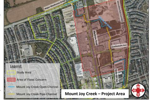
that reduce frequent overland flooding of the properties adjoining the creek corridor, improve conveyance, and must be sufficient to facilitate the future development ambition for the area defined in the recently completed Markham Road Mount Joy Secondary Plan. A total of eight (8) potential drainage alternatives were developed and presented at PIC #1. These alternatives have now been hydraulically modelled and evaluated based on a total of four (4) Evaluation Criteria including;
