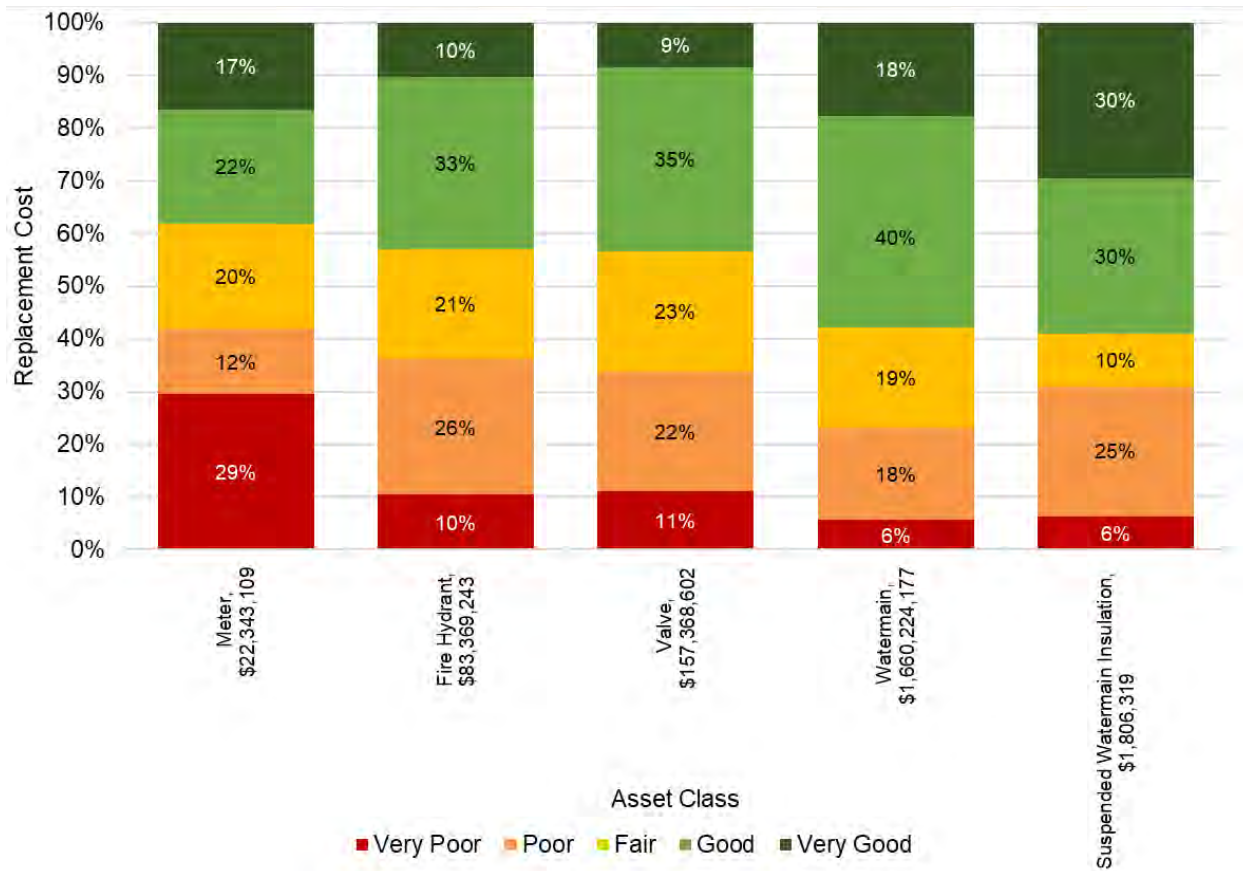
Figure A - 7: Condition distribution of Potable Water assets by asset class.
