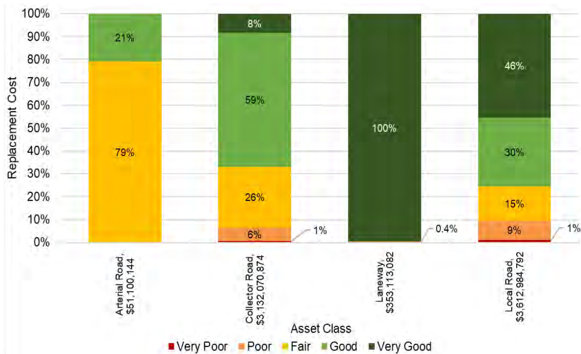
Figure D - 10: Condition distribution of Vehicular Transportation assets by asset class (roads only and based on PCI ratings).
