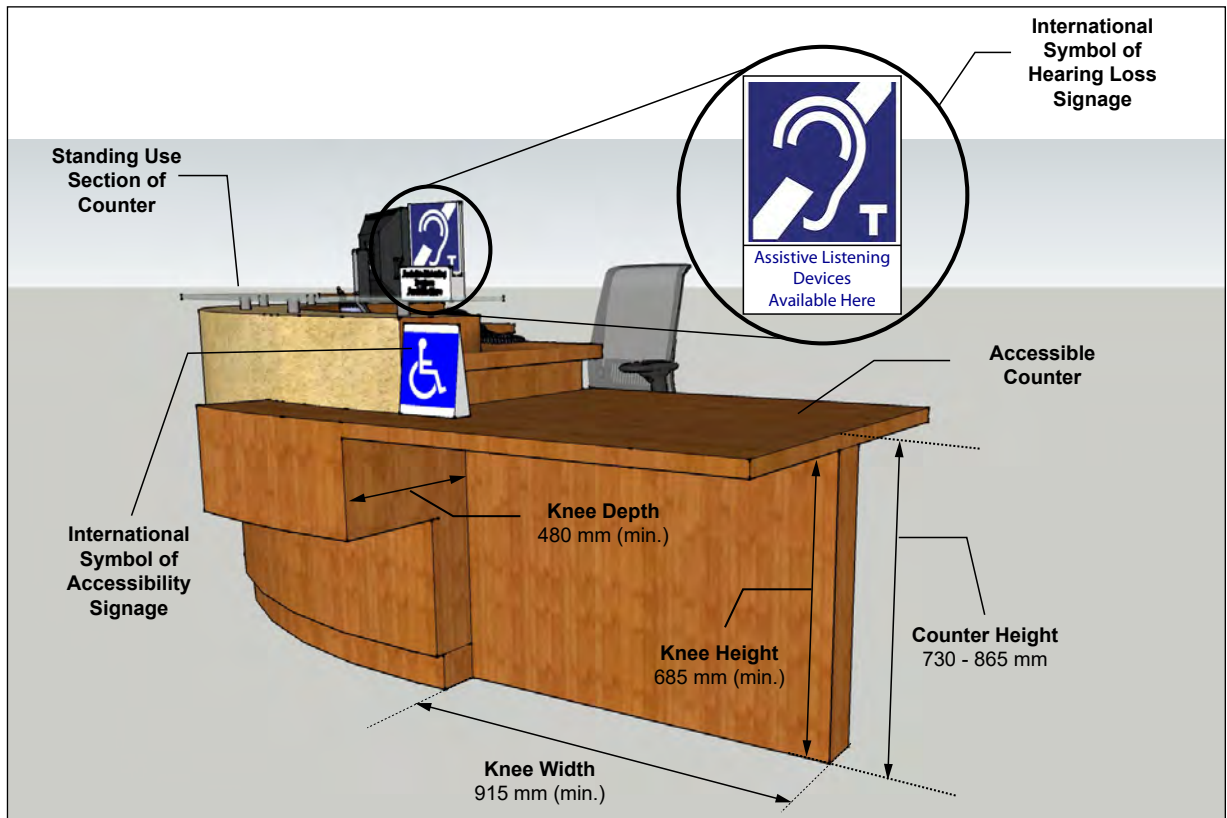
Figure 97b: Accessible Service Counter with Knee Clearances
