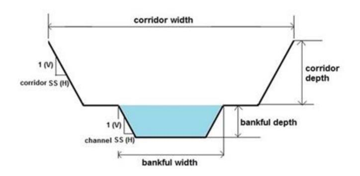
Figure 5. Schematic example of modelled cross-section.
