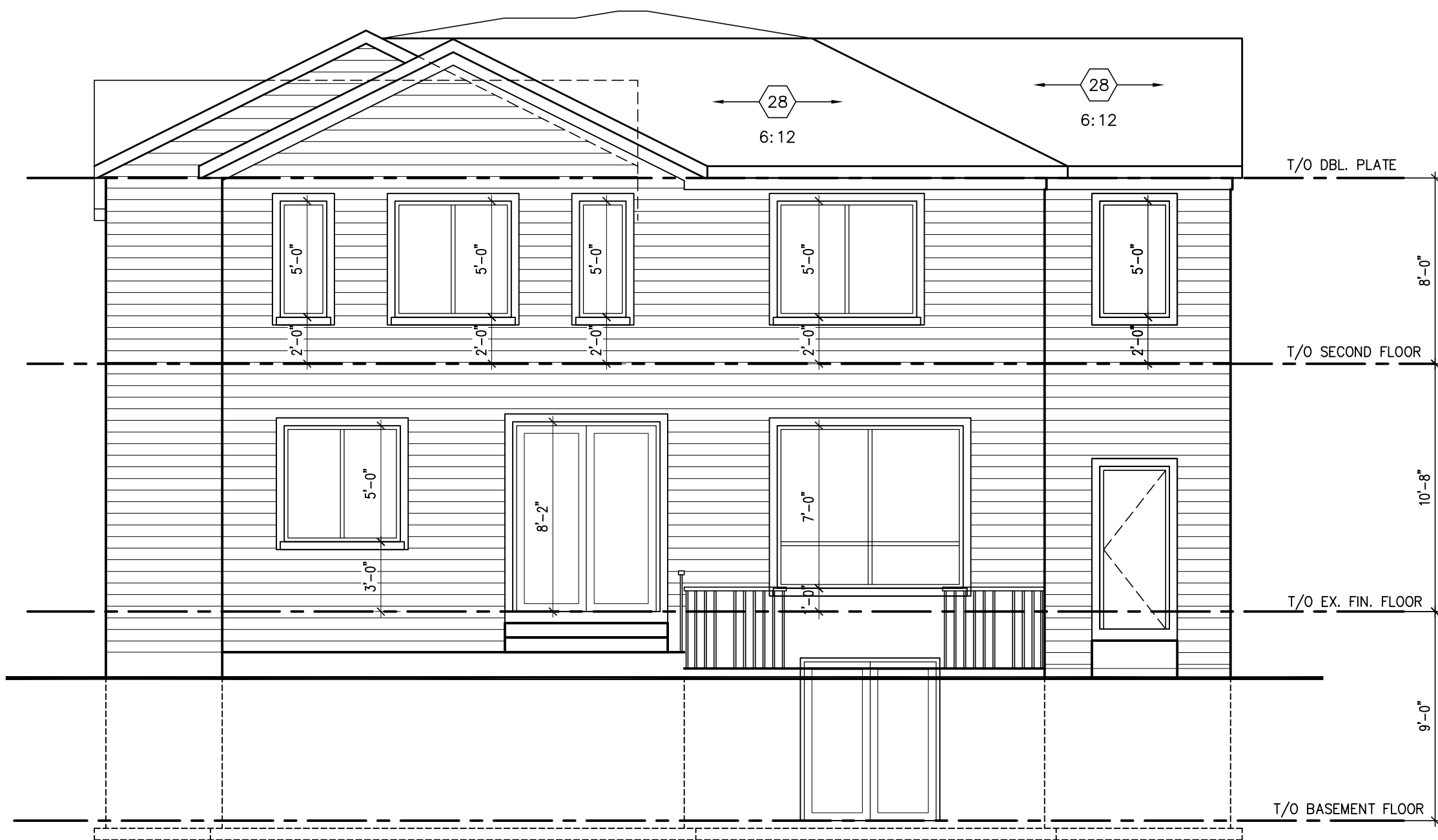
3 WEST SIDE ELEVATION SCALE: 3/16"=1'-0"
