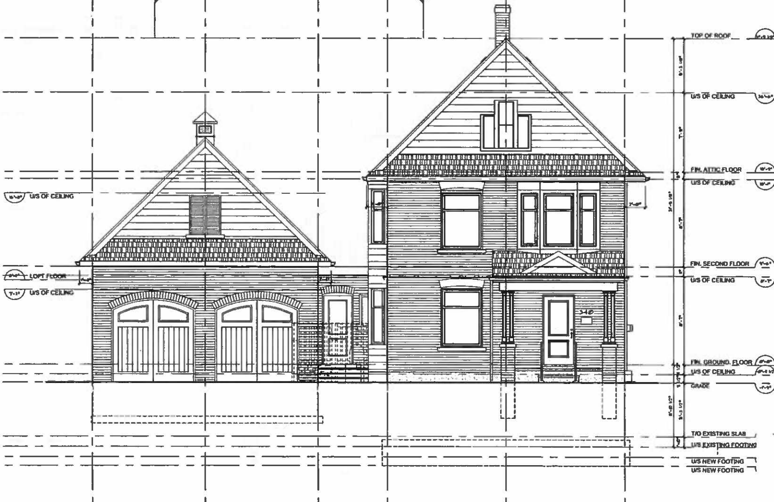
FRONT (EAST) ELEVATION AS PROPOSED Scale: 1/4" = 1'-0"
