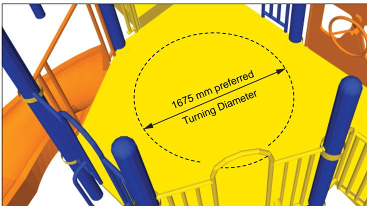
Figure 102: Turning Space - Plan View
