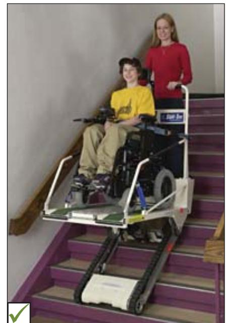
Example of portable elevating device, with platform designed to accommodate mobility aid during evacuation.
