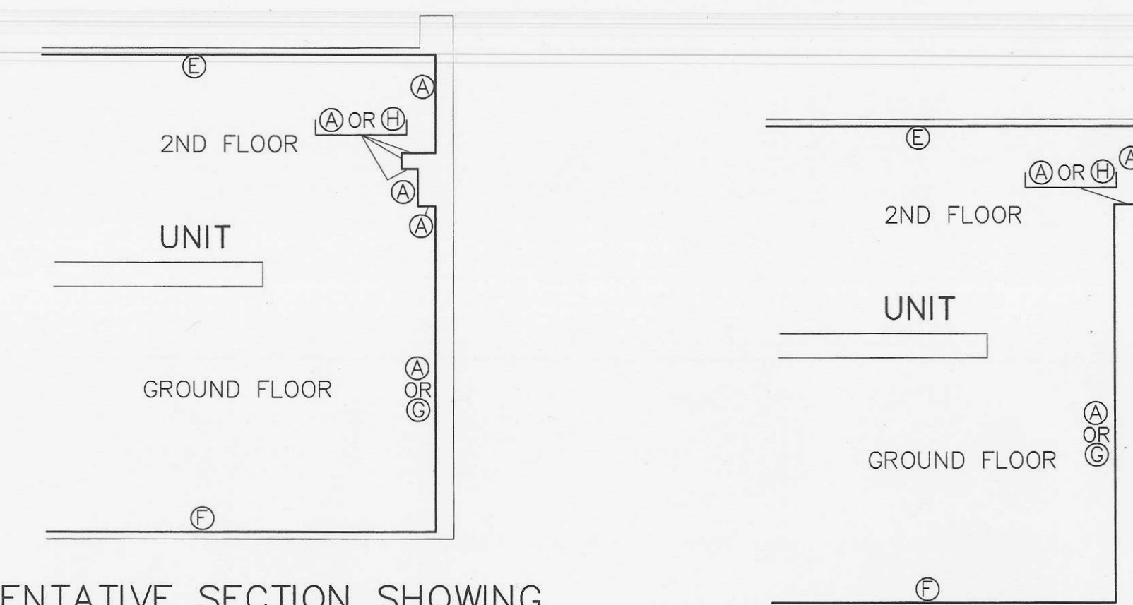
REPRESENTATIVE SECTION SHOWING TYPICAL UNIT BOUNDARIES AT THE REAR OF UNITS 98, 99, 100, 101, 106 AND 112 (NOT TO SCALE)
