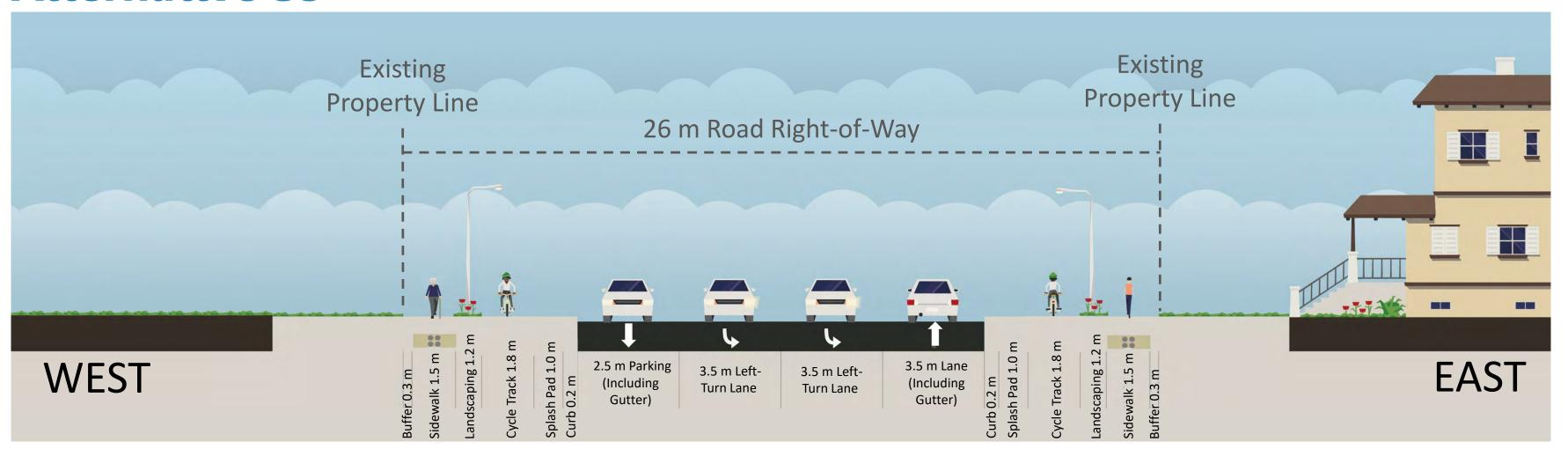
Note: Where constraints exist, the separate sidewalk and cycle track facilities may be combined into a single multi-use path facility. Details would vary by segment.
